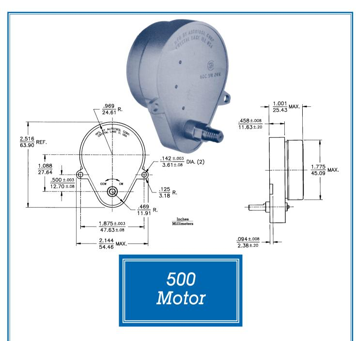
A powerful permanent magnet synchronous motor in a very compact package. Delivers 500 ounce-inches of torque at 1 RPM. Speeds available from 1/2 RPM to 240 RPM. Suitable for many instrument and industrial applications.
