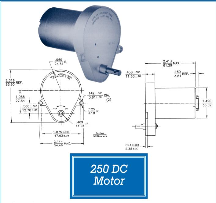
The 250 motor is a permanent magnet gearmotor utilizing barium ferrite 2 pole field magnets. Carbon brushes provide long life, quiet operation and low starting voltage. The rotor is supported by permanently lubricated sintered bronze bearings. The 250 motor is available in a wide range of speeds and is an excellent choice for applications requiring reliability and quiet operation at low cost.
